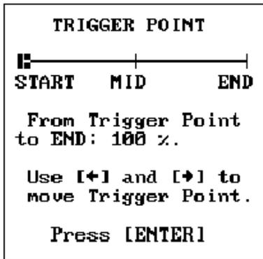
The display at the left stores 100% of the data after the trigger point.
