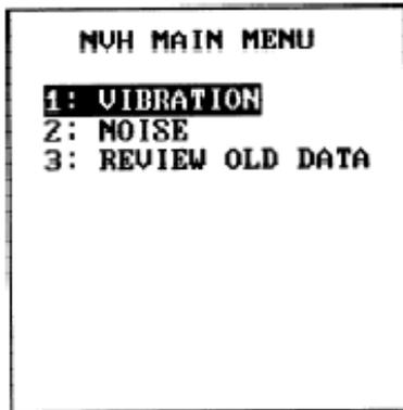
In the <NVH MAIN MENU>, all functions available for the selected system are displayed. To select a function, press the key to the left of the function you wish to use. The use of each function is explained on the following pages.
