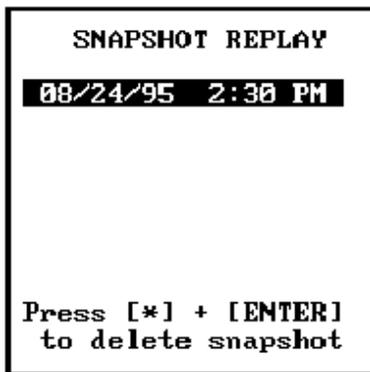
Press **(3)** to select <SNAPSHOT REPLAY> mode from the <GAS ANALYZER> menu. Snapshot Event Replay options are listed below:
